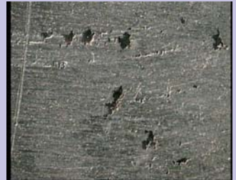
Pits on AA5083-H116 after 24 hrs in NH 4 Cl+NH 4 NO 3 +(NH 4 ) 2 C 4 H 4 O 6 +H 2 O 2 solution. X10
